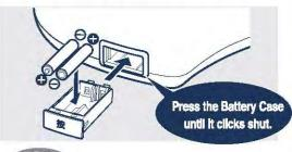
●Be sure to set the polarity ( + - ) of the batteries correctly.
