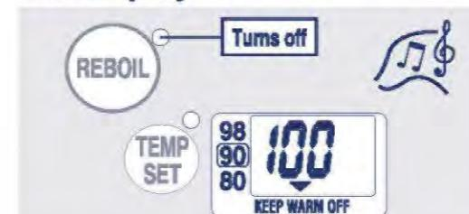
When the boiling process has completed, a melody sounds and the BOIL light turns off.
