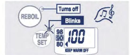
When the boiling process has completed, a melody sounds, the BOIL light turns off, and the KEEP WARM light begins to blink.
