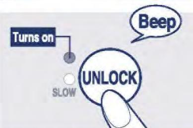
The **UNLOCK** light turns on and hot water can be dispensed.
